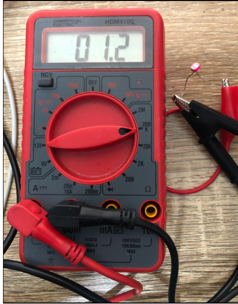
Figure 74 - Using Laser Diode as Light Source Measuring Resistance
