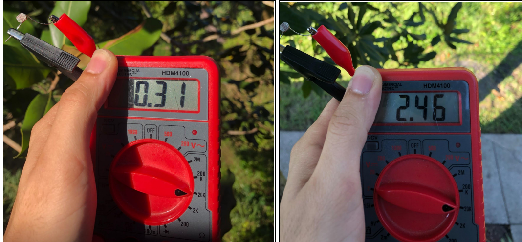
Figure 76 - Outside LDR Testing in Direct and Indirect Sunlight
